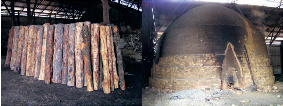
Figure 4-3 Mangrove timbers (left panel) were transferred and sealed in a special-designed kiln (right panel) to produce charcoal using a process called pyrolysis. (Photo by Ooi AL)
